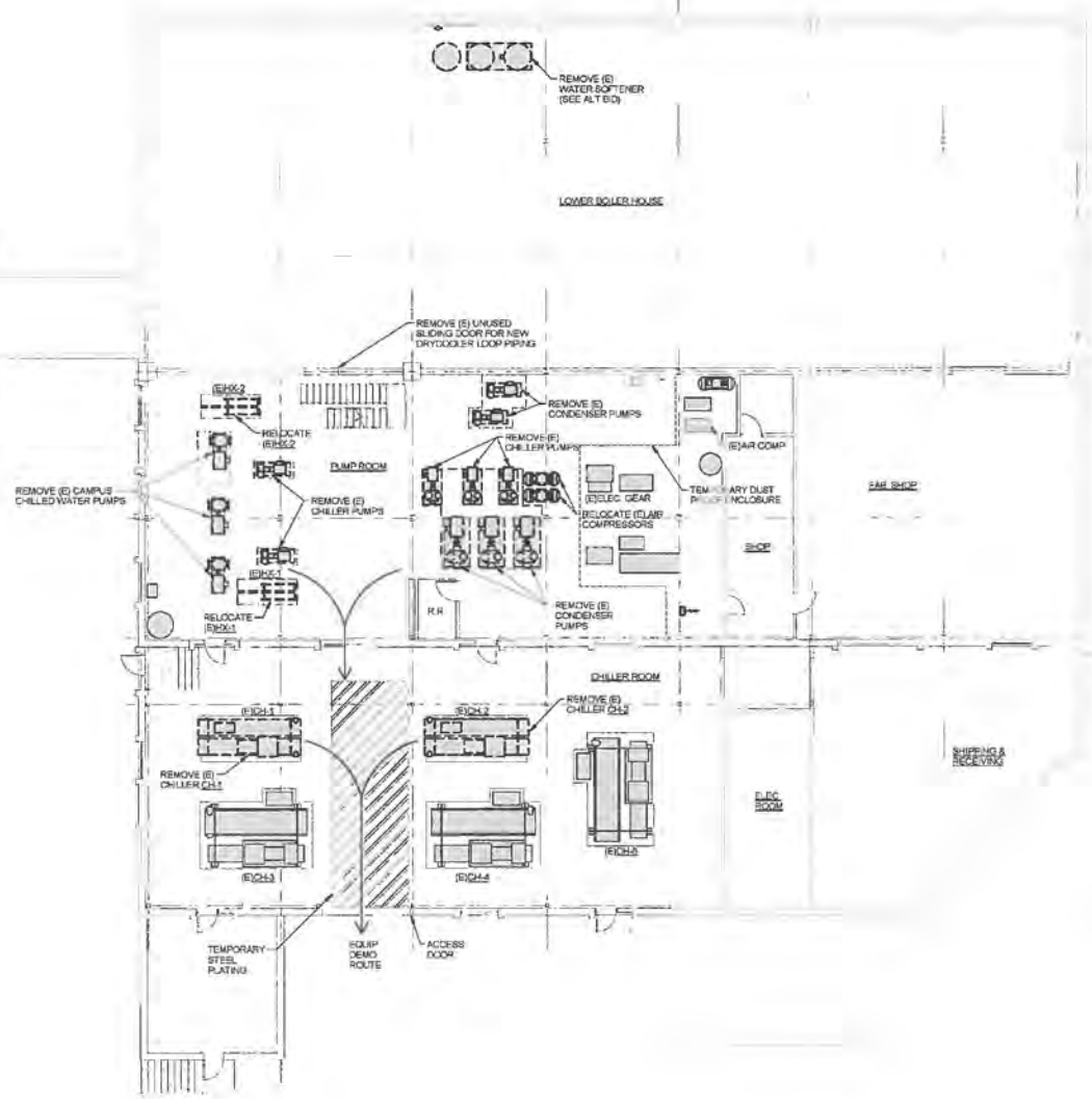
Z 1 GROUND LEVEL - OVERALL PLAN - MECHANICAL DEMOLITION (SEE M3-2.1 THRU M3-2.9 FOR DETAILS) SCALE: 3/32" = 1'-0"
