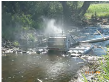
Fish screen installed on a pump diversion in a creek.
