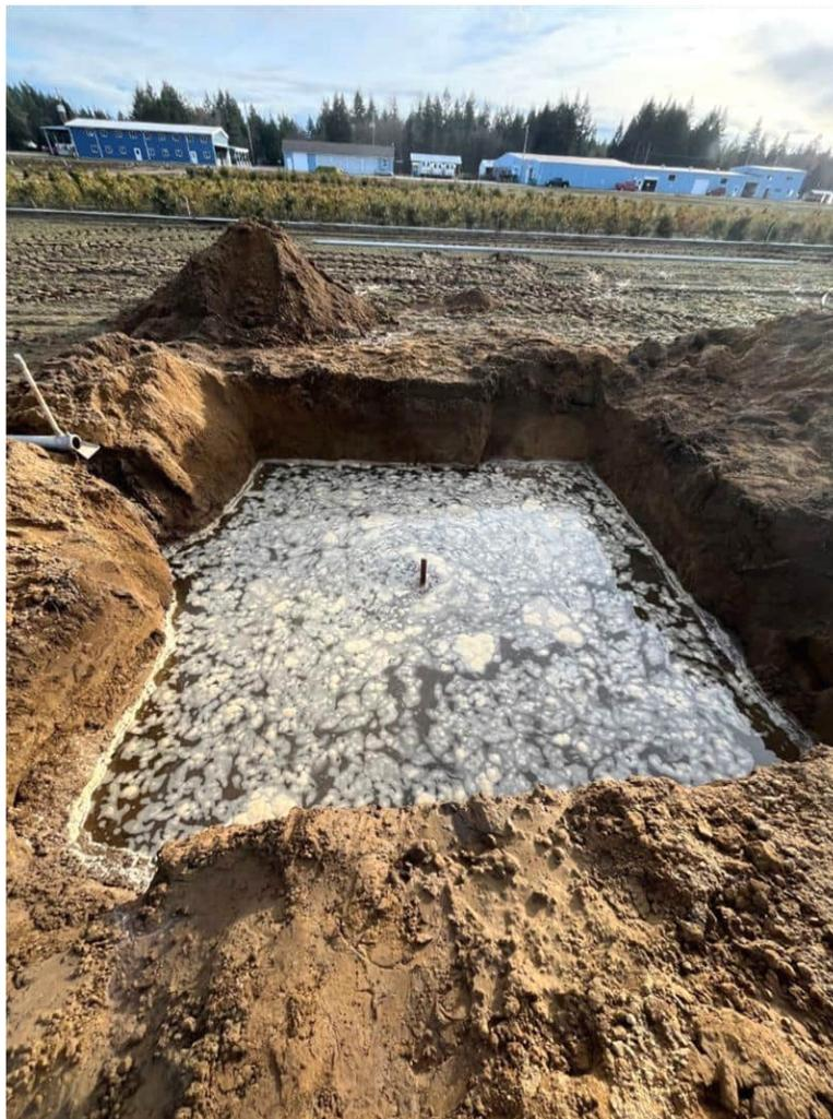
*Photo 4 – TP-6 at start of steady infiltration monitoring.*
