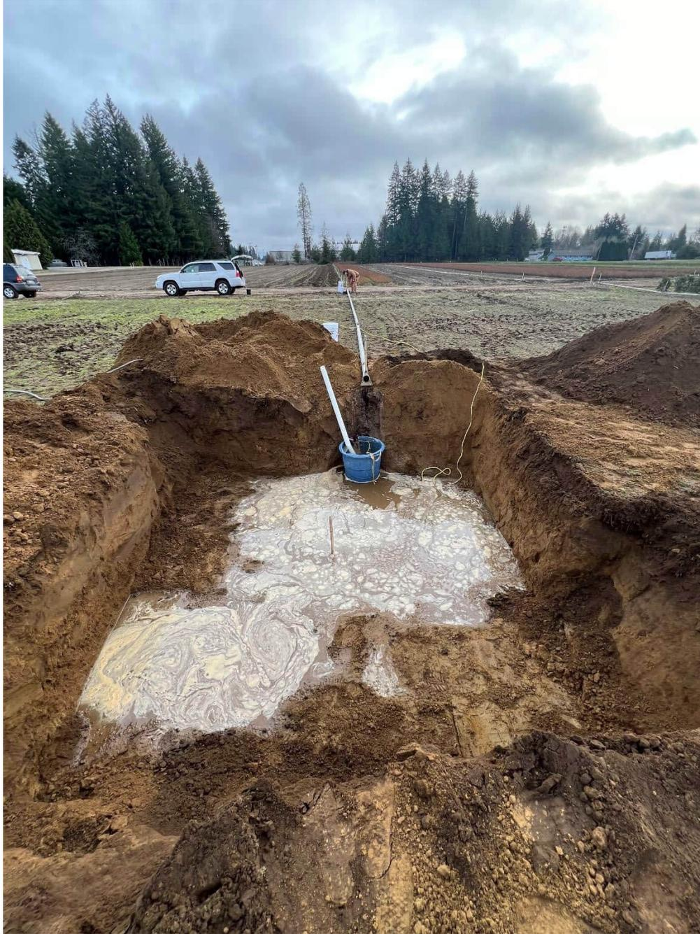
*Photo 2 – TP-6 at the start of infiltration testing – pond filling.*
