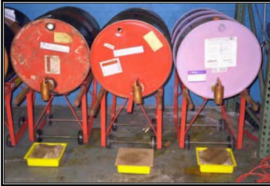
**Figure IV - 4.18 Mounted Containers with Drip Pans.**
