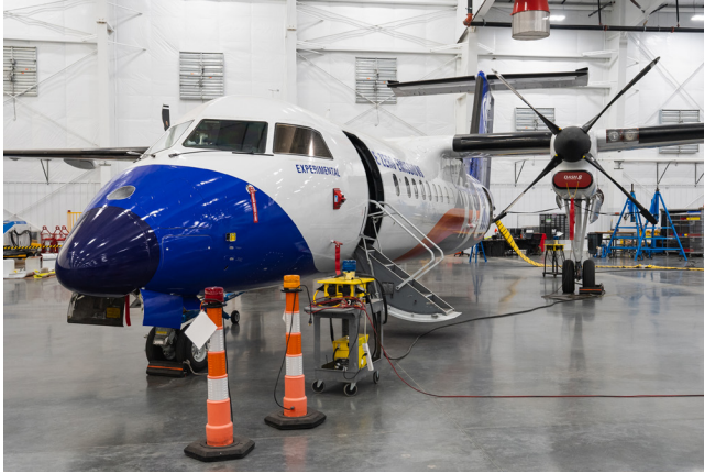
This De-Havilland Dash 8-300, the largest hydrogen-powered plane yet to fly, at Grant County International Airport. The plane is propelled by an electric motor developed by Everett-based magniX running on a hydrogen fuel cell system developed by Spokane Valley-based Plug Power. The airframe is already in popular use; the experiment shows that sustainable aircraft are very nearly ready for commercial use.
