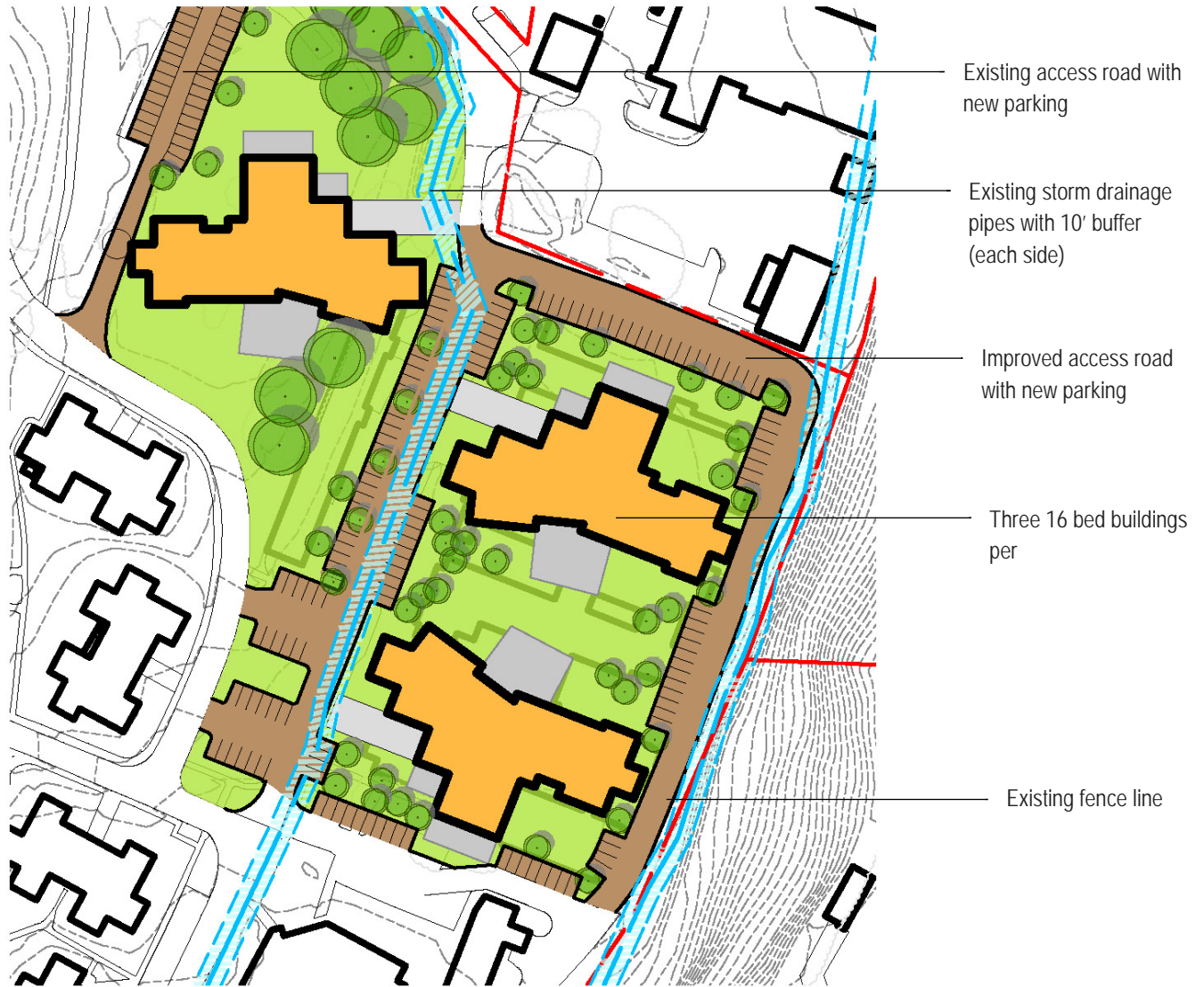
Figure 24 Diagrammatic site plan for a behavioral health center in the Northeast Corner (Area 1)
